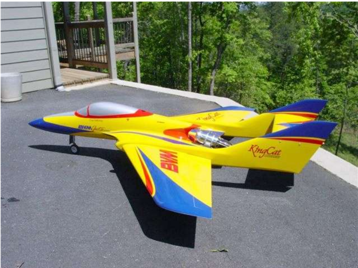
Photo 10 – Finished King Cat. It weighed in balanced right at 27 pounds. The extra weight of the smoke system perfectly offset the slightly heavier AMT-280 turbine.
